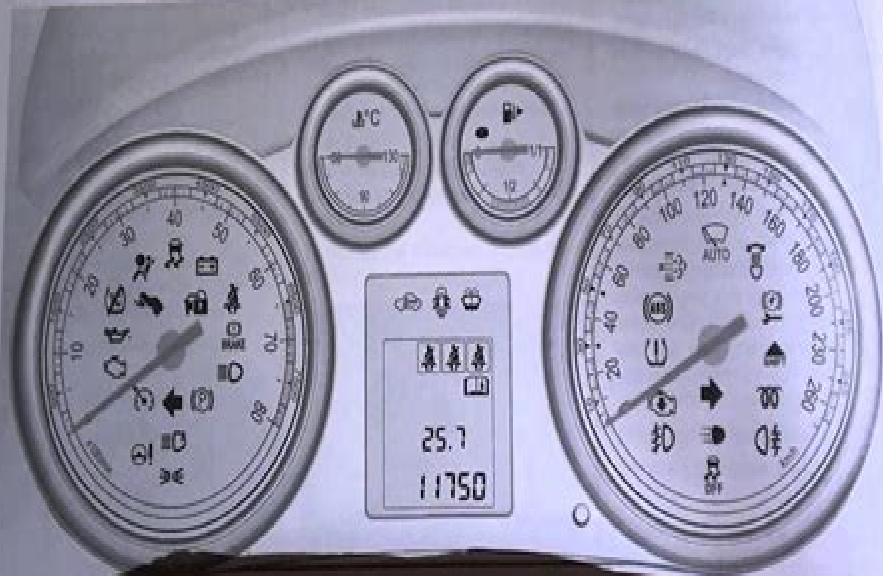
Control indicators in the instrument cluster
