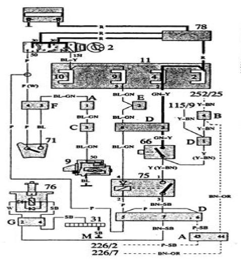
**legition** switch Starter motor 11 Electrical distribution unit 31 Ground/earth busbar in electrical distribution unit 66 Brake light switch 71 Start inhibitor 75 Relay, shift lock 76 Solenoid, shift lock 78 Positive terminal 115 **Bulb failure warning sensor** 226 Control unit, cruise control 252 Control unit, ABS
