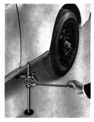
Insert jack into socket and push the jack tube down until it touches the ground.
