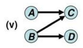
C cannot begin until both A and B are completed; D cannot begin until B is completed. A dummy activity is introduced in AOA
