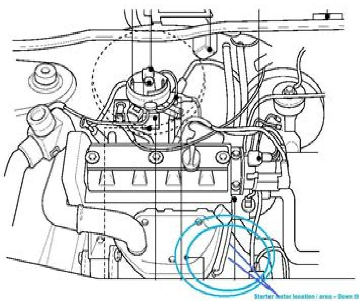
Starter Nator location / area - Down the front of the engine - builted to the gearbox.....
