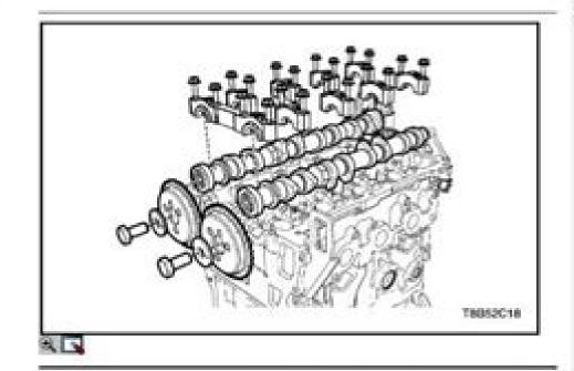
Install the camshaft. Refer to "Unit Repair-Camshaft" in this section.
