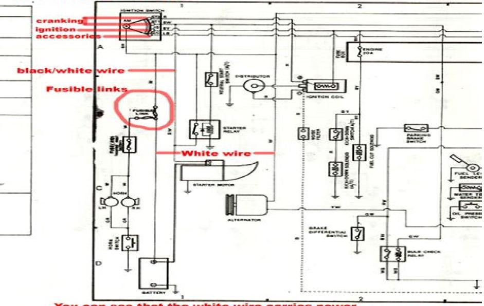
You can see that the white wire carries power from battery to ignition. The B/W powers the starter solenoid.
