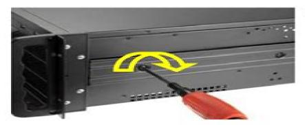
Unscrew all three screws on each side.
