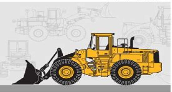
Engine output SAE J1995; power, gross 259 kW (352 hpl) 15/0 9245 SAE 21349: power, net 297 kW (349 hpl)
