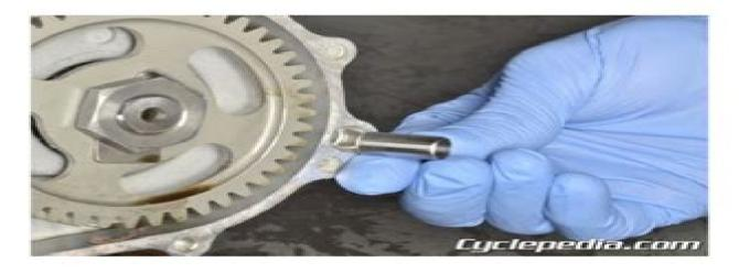
Remove the right crankcase cover gasket and two dowel pins.
