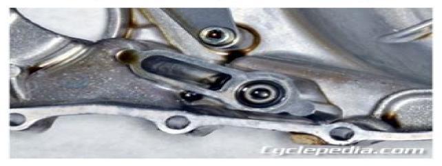
Inspect the oil pressure relief valve in the right crankcase cover. The steel ball should move smoothly when pressed in and return to its resting position without sticking.
