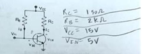
Transistor Feedback Biasing
