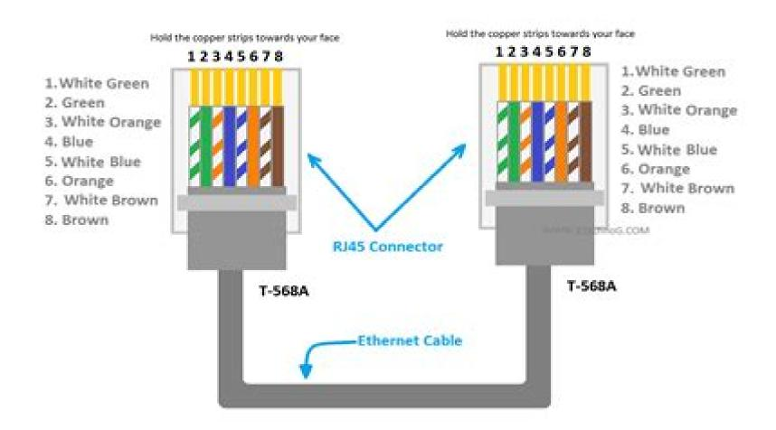
Ethernet Wiring Diagram with Color Code Guide
