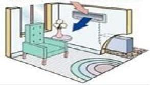
ALL YOU NEED IS A 3 INCH HOLE IN THE WALL TO RUN THE CONNECTION BETWEEN TWO UNITS
