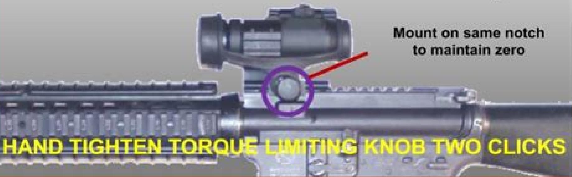
HAND TIGHTEN TORQUE LIMITING KNOB TWO CLICKS
