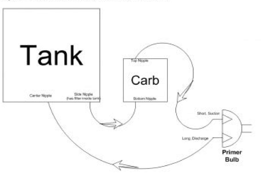
Ryobi 770r fuel line connections: Note: the primer bulb pulls fuel from the carb and pumps it back to the fuel tank. This causes a vacuum in the carb that draws fuel from the tank to the carb through the filtered fuel line.
