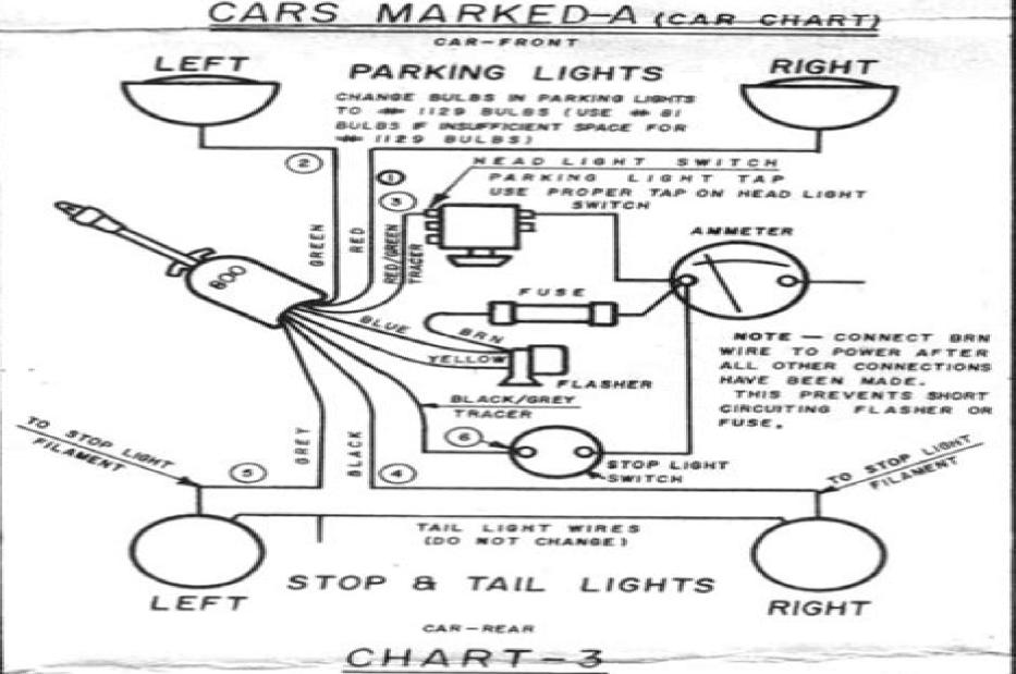
SHOWING "SIGFLARE" WIRED TO LAMPS, SWITCH TERMINALS AND FLASHER WIRED TO AMMETER.
