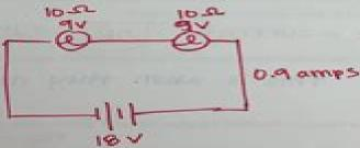
Current: 0.9 Total Voltage: 195 Total Resistance: 20 Brightness of Bulbs (scale of 1 to 3): 2 Calculations:
