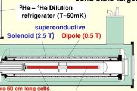
2002-2004: <sup>6</sup>LiD dilution factor f = 0.38 polarization P<sub>T</sub> = 50% ~20% of the time transversely polarised
