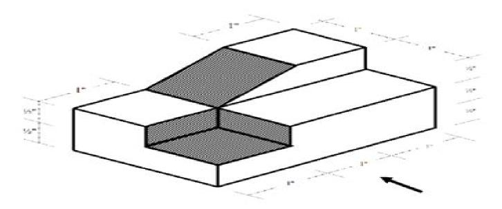
Assignment No 7: Draw the isometric view of the figure below. Maintain proper margin and title box mentioned in the class. (The arrow indicates the Front view).
