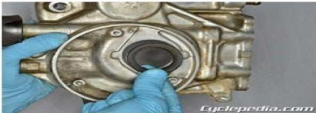
Inspect the crankshaft oil seal and replace it as needed.
