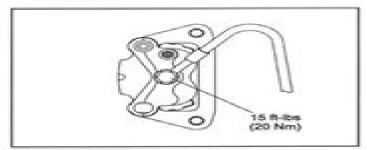
Install the adjustment set screw and turn clockwise until stationary pad contacts disc, then back off 1/2 turn (counterclockwise).
