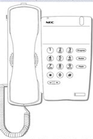
C Analog Single Line Telephone is displayed here. This guide a general analog phone procedures. Refer to the user guide included ar specific analog phone for details on additional key functions.
