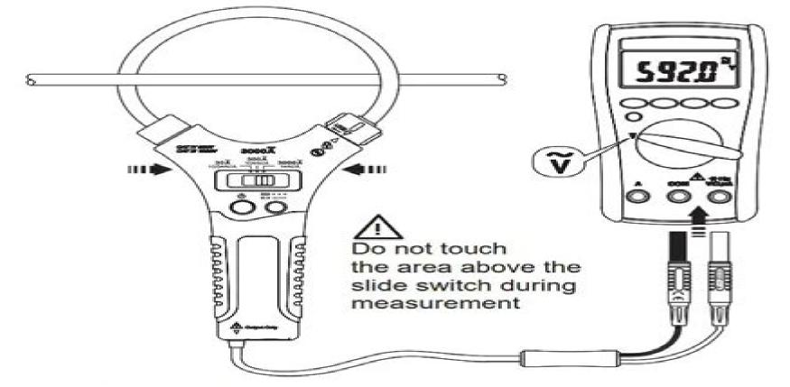
Set DMM at AC 3.000V range and switch sFlex-T to the suitable range. Calculate the correct current according to "AC Current" specifications.
