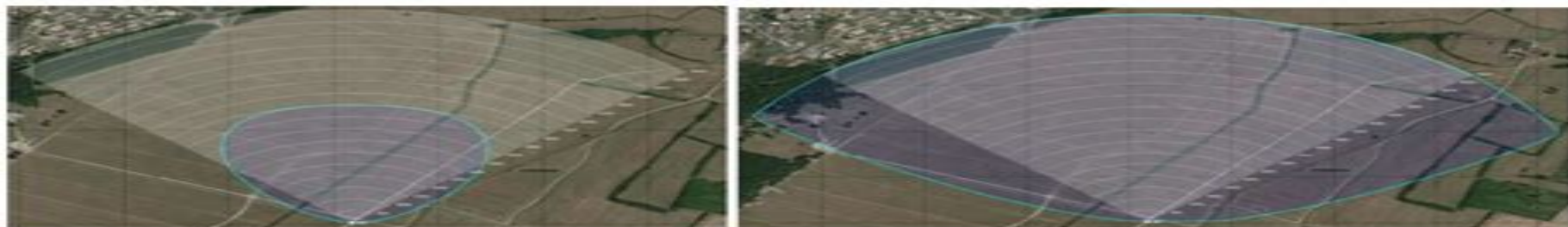
Figure 46: Detection zone for a human intrusion (left) and for a car (right)
