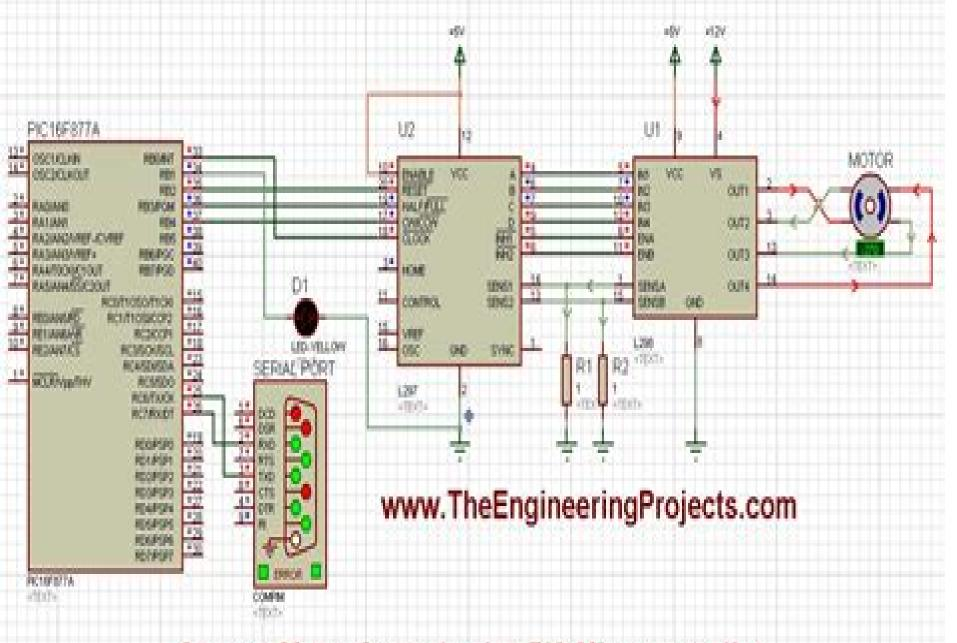
Stepper Motor Control using PIC Microcontroller
