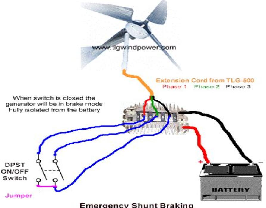
**Emergency Shunt Braking**
