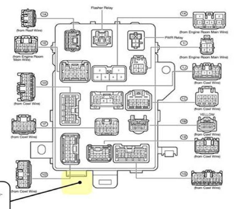
Circuit Opening Relay here (bottomright if looking straight on from drivers side)
