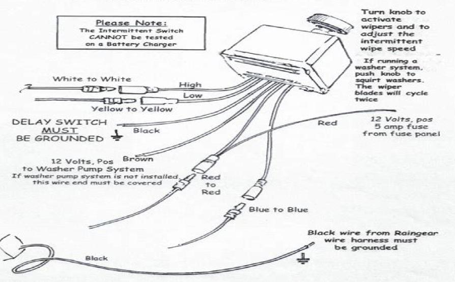
NOTE: The colors of the wires from the wiper motor and the colors of the wires on the harness do not match. This is correct.
