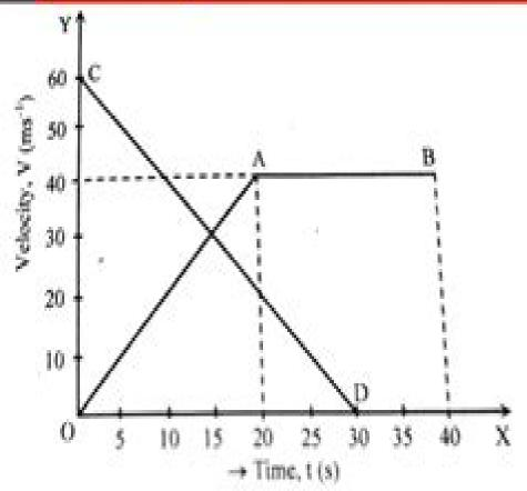
The graph shows velocity vs time. From the graph OAB line for the first car and CD line for the second car.
