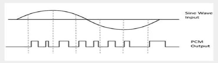
Instead of a pulse train, PCM produces a series of numbers or digits, and hence this process is called as **digital**. Each one of these digits, though in binary code, represent the approximate amplitude of the signal sample at that instant.
