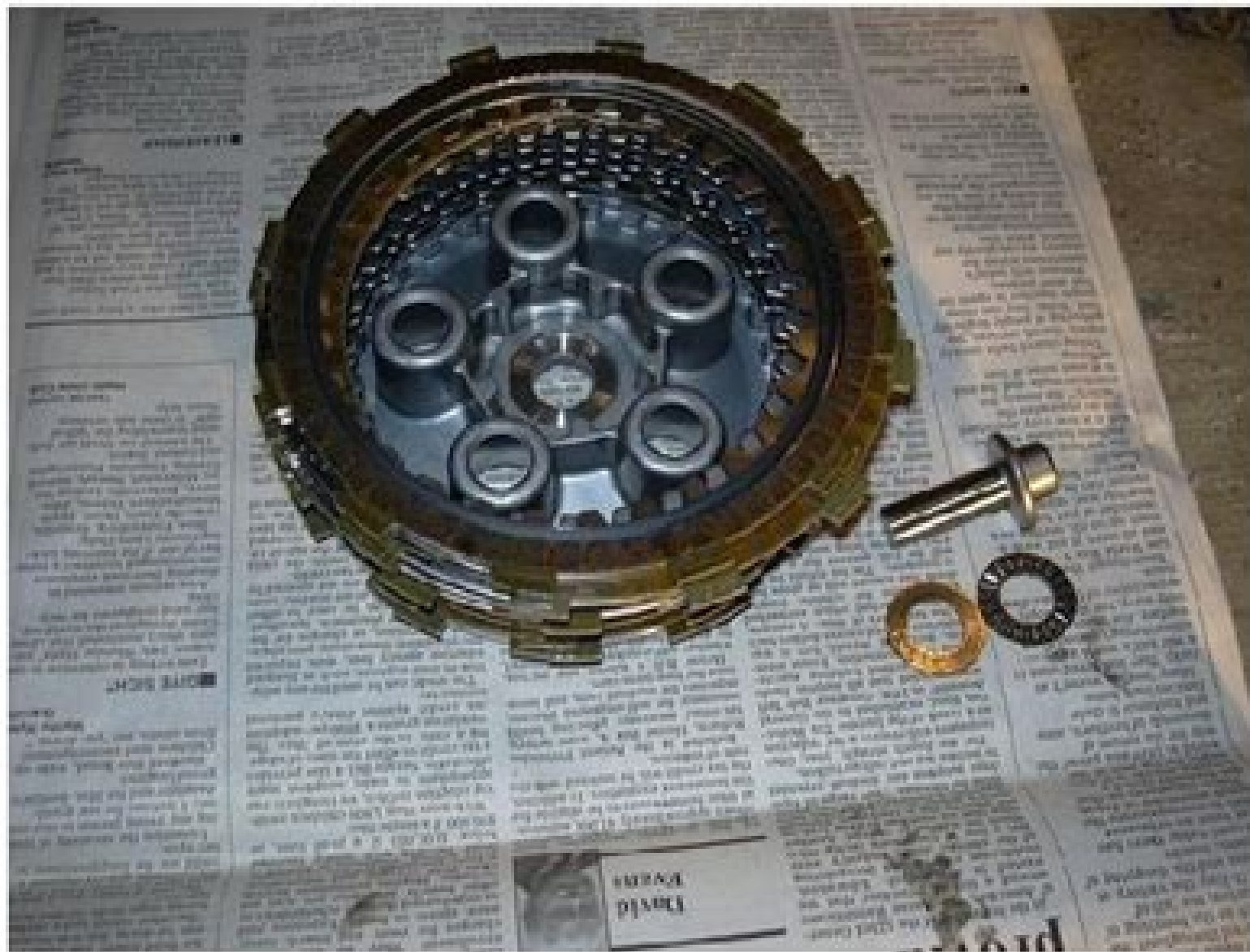
Removed clutch plates (drive and driven) stacked in order on the pressure plate, note the clutch rod top hat, thrust bearing, and thrust washer. Keep all from dust and dirt.
