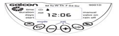
Press ⊕. The minute digits blinks. Set the current minute with the aid of ⊕ or ⊡.
