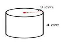
A cylinder has a circular base. Use  $A = \pi r^2$  to find the area of the base.
