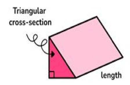
Volume of a triangular prism = Area of triangular cross section  $\times$  length
