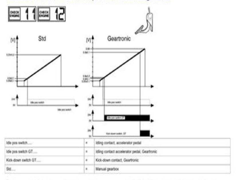
The diagram on the left shows the normal voltage rangeand the correct engagement position for the iding contact in a vehicle witha manual gearbox.
