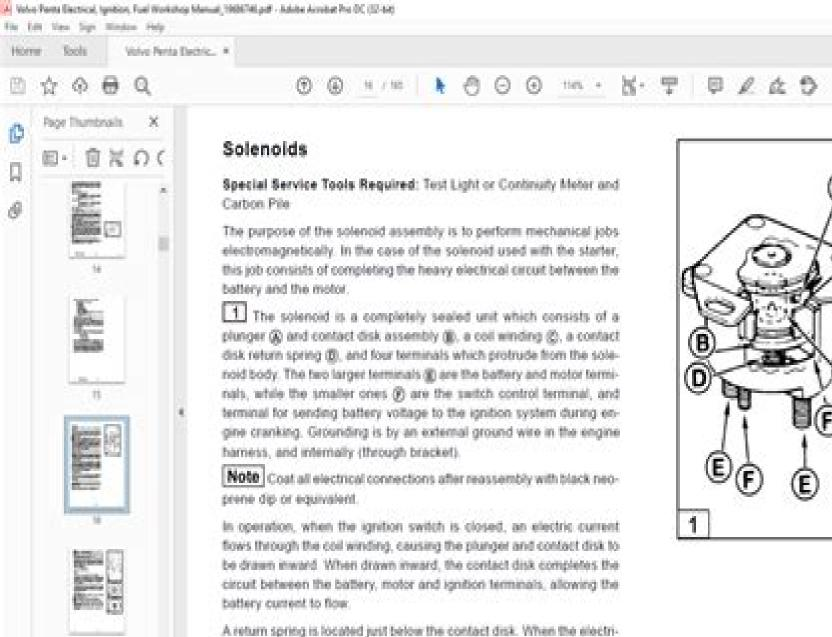
A return spring is located just below the contact drisk. When the electrical circuit as described above is completed, the spring is compressed by the magnetic pull on the plunger and contact disk. When the electrical circuit is broken (ignition switch released), the magnetic pull on the plunger and contact disk drops to zero. At this time, the compressed
