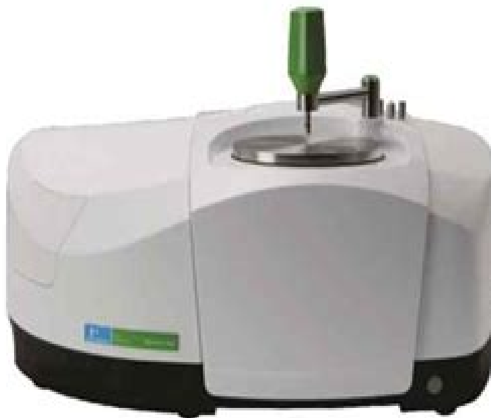
Figure 8 Spectrum Two FT-IR with Universal ATR Accessory
