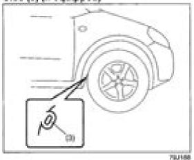
Frame hooks are provided on the front (1), rear (2) and side (3) (if equipped) of the vehicle. The hooks (1) and (2) are used for emergency situations. The hooks (3) (if equipped) are used for trailer/train shipping purposes.
