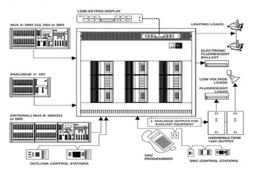
All power blocks are fitted with MCBs, and an RCD may be included as an option. Racks may be positioned and cabled before the power blocks are installed, to reduce the risk of damage during building work. Each power block has the same overall size and power requirement, so a mixture of 2.5kW and 5kW dimmers may be included in the same rack. Blank power blocks are available for custom equipment or branch breakers, or just for completing a partly-equipped rack.
