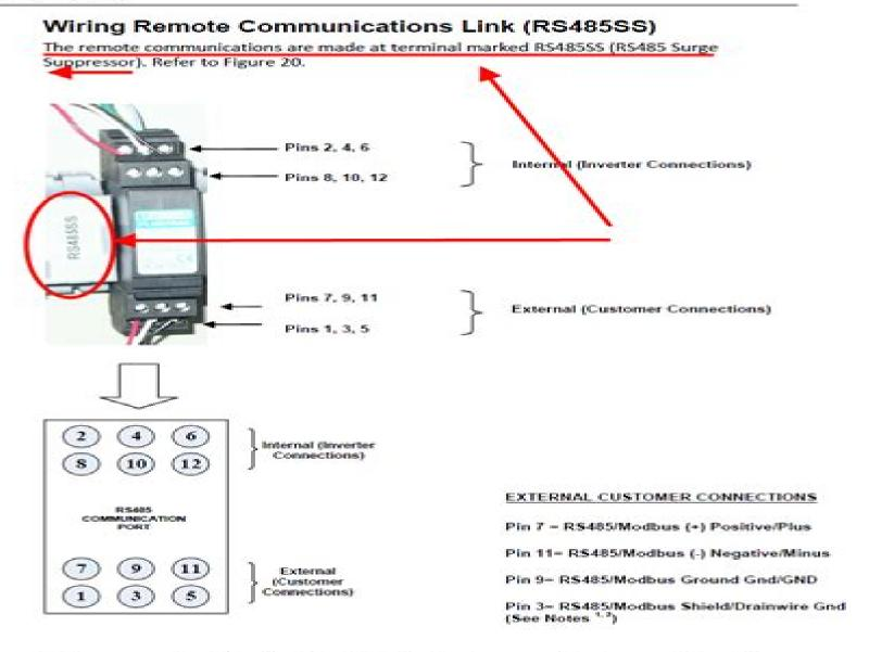
Only connect the drain wire of the shielded cable at one end. Do not ground the drain wire at both ends of a cable run or connection hookup.
