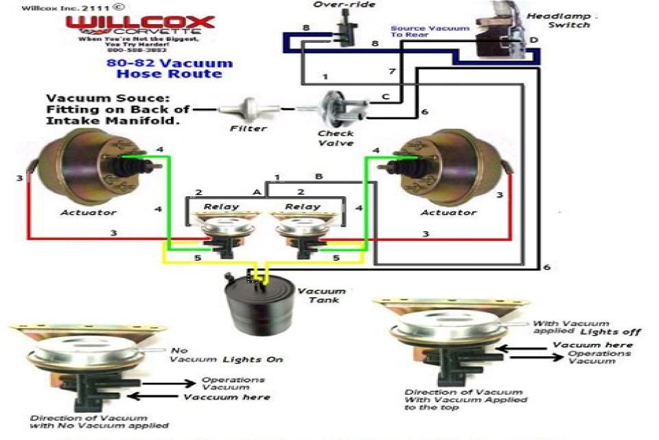
The vacuum Actuator relays operate the up and down movement of the item controlled either the windshield wiper door or the headlamp actuator. Consider this relay as the up and down switch controlled by vacuum at the top. The larger top nipple is the pull down side and the lower large nipple is the pull open side all controlled by the smaller metal nipple on top.
