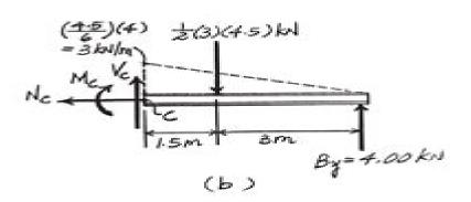
Ans:  $N_C = 0$ ,  $V_C = 2.75 \text{ kN}$ ,  $M_C = 7.875 \text{ kN} \cdot \text{m}$
