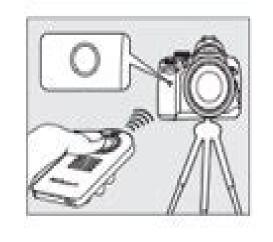
If no operations are performed for about five minutes after selecting delayed remote or quick-response remote modes, the camera will automatically return to single frame or continuous mode, cancelling remote control mode.
