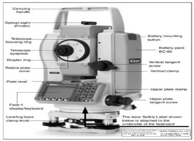
Figure 1.1 Pulse Laser Station NPL-302 series - Face-1
