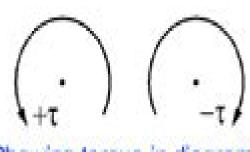
Showing torque in diagrams
