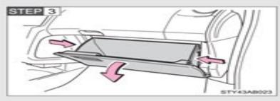
Push in each side of the glove box to disconnect the claws.
