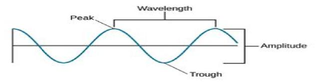
Wavelength is directly related to the frequency of a given wave form. Frequency refers to the number of waves that pass a given point in a given time period and is often expressed in terms of hertz (Hz), or cycles per second. Longer wavelengths will have lower frequencies, and shorter wavelengths will have higher frequencies ([link]).
