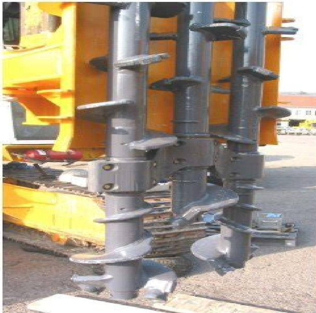
Mixing self-hardening slurry in-situ with native soil (SMW) is a cost-effective technique for the construction of walls for groundwater control (cut-off walls), walls for excavation support (retaining walls) as well as for ground improvement.
