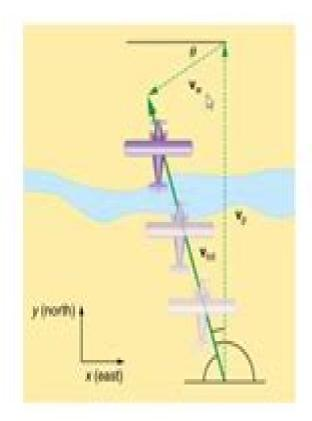
An airplane heading straight north is instead carried to the west and slowed down by wind. The plane does not move relative to the ground in the direction it points; rather, it moves in the direction of its total velocity (solid arrow).
