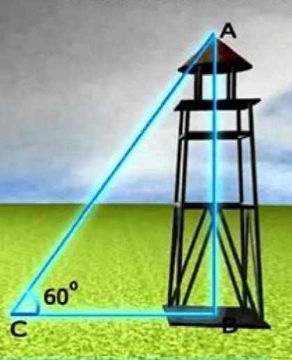
∠ACB is the angle of elevation
